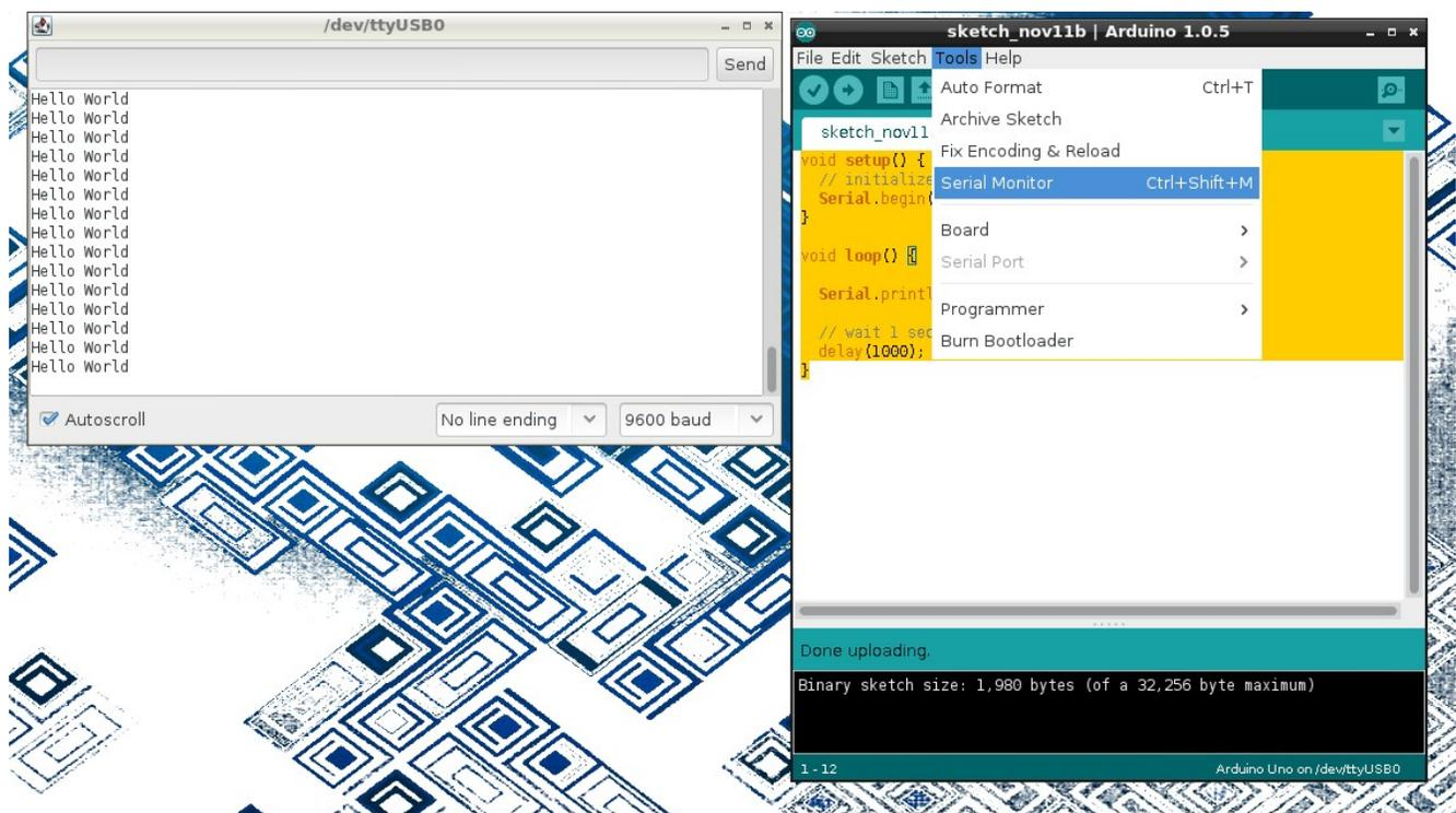
**Serial.begin(9600);** opens the serial port at on the Arduino and sets its speed to 9600 baud
