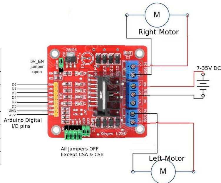
The polarity of the motors (motor-a +, motor-a -) doesn't even really matter as the opposing motor will probably be turned around (180 degrees), so for your application you simply change the HIGH/LOW signals you send the IN1 and IN2 board inputs and that toggles the motor direction. Here's the example code for driving the motors:
