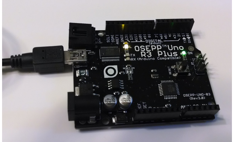
Illustration 1: Arduino Clone with power and "blink" light
