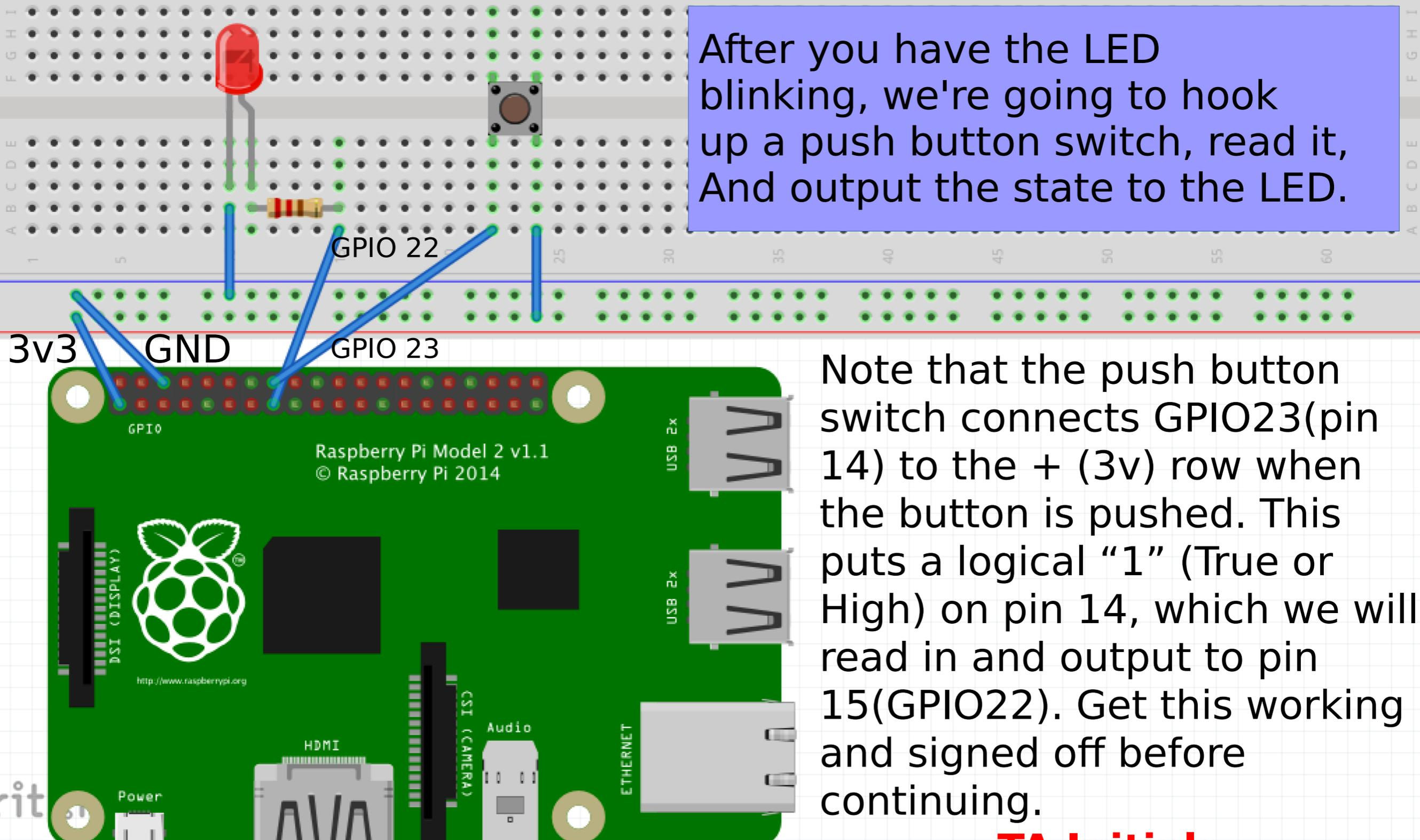
Note that the push button switch connects GPIO23(pin 14) to the + (3v) row when the button is pushed. This puts a logical "1" (True or High) on pin 14, which we will read in and output to pin 15(GPIO22). Get this working and signed off before continuing.
