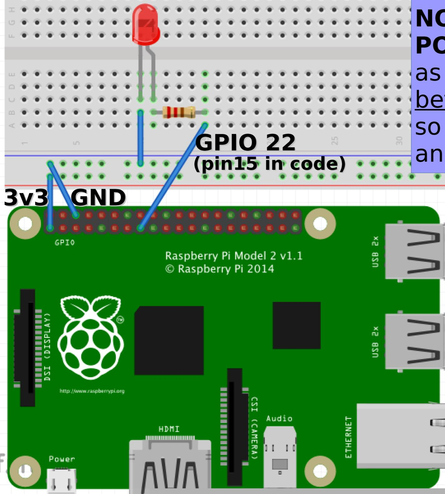
Here's how to hook up the Pi (GPIO22=pin15) to your breadboard and LED. Note that your kit may have a big rainbow ribbon cable and "T" shaped board connecting your Pi to the breadboard. Do not go beyond this section until you have it working.
