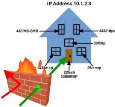
As seen in the image (right), a firewall is a piece of hardware or software that is designed to block and allow traffic based on who (or what IPs) are trying to get in on specific service ports. Allowing a port or source IP through a firewall is casually called "poking a hole" (granting access), as illustrated in our house IP address image.
